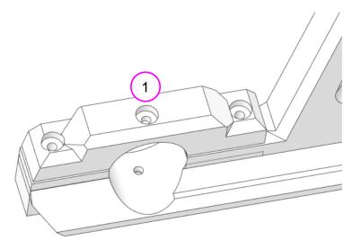
5. Fit both rudder mounts to the motor mount with M3 x 10 mm self-tapping screws.
