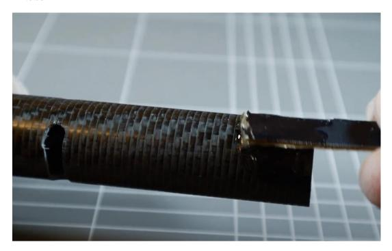
10. Then slide the tube mount on to the 25 mm x 575 mm carbon fibre tube and use M5 x 60 mm socket head bolts to position it correctly. Repeat the process for the other end of the 25 mm x 575 mm carbon fibre tube and tube mount. Pay particular attention to ensure that both tube mounts are orientated correctly.
