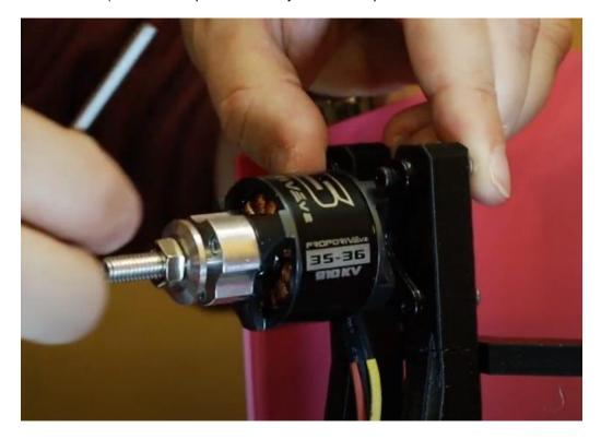
4. The motor mounts and brackets have a hole (1) centred on the carbon fibre tube. Drill these holes at 90° through the carbon fibre tube. There is no need to offset the angle of the motor mount to alter the hull's pitch as this can be done using spacers when mounting the motor if required later on. Fit M3 nuts in the bottom of the motor mount braces and then secure the mounts through the tube using M3 x 40 mm machine head screws.
