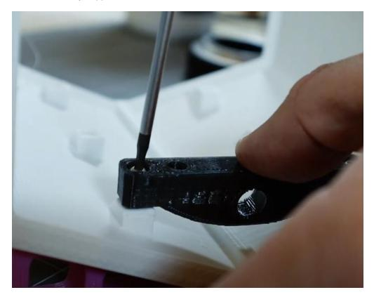
3. Install M3 x 4 mm heat-set inserts into the tray mounts.
