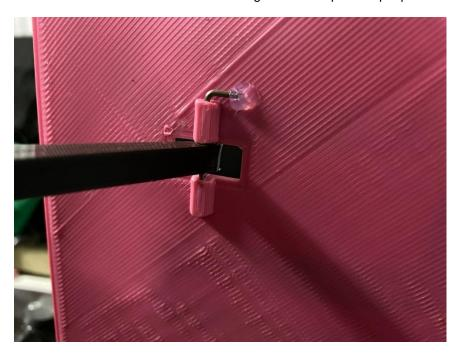
8. Insert M3 x 4 mm heat-set inserts using a soldering iron into the holes (1) in the bottom of the servo mount.
