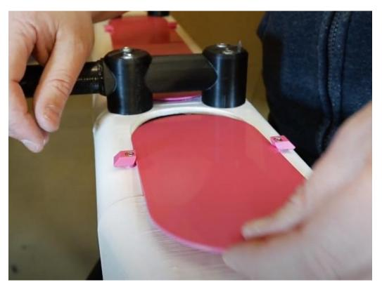
14. The rear hatch must be assembled in two pieces as per the image below so that it can fit between the tube mounts.
