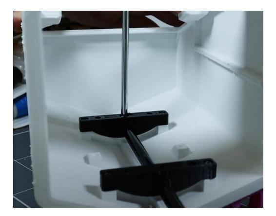
5. Using **2-part epoxy glue** (JB Marine Weld is recommended), join each of the sections together by passing them onto **8 mm x 600 mm carbon fibre tube** one by one. You will need to work quickly before the epoxy goes off.
