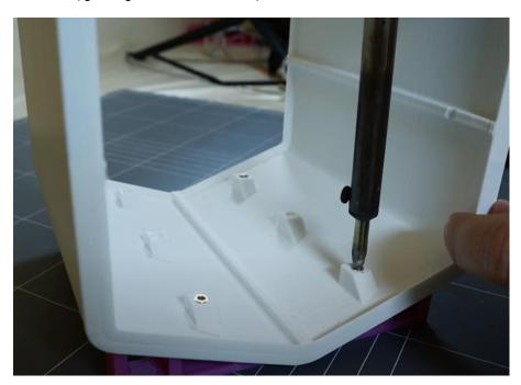
2. Install the tray supports into the hull with  ${\bf M3~x~12~mm~machine~head~screws}.$
