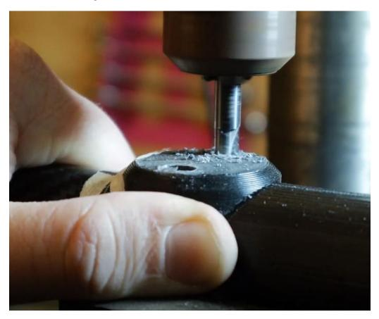
8. When milling, pass **M5** x **60** mm socket head bolts through the holes (1) to act as an end stop for the carbon fibre tube. Only mill the carbon fibre tube through the holes (2).
