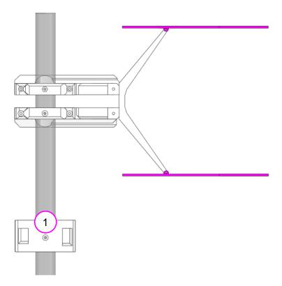
10. The servo mount suits a standard sized servo. A waterproof servo is recommended. Fit your servo using the included mounting hardware (not included in bill of materials). The image below shows the rudder linkage in place. The rudder spacer is fitted by drilling a 3 mm hole in the rudder and using control horn hardware to secure it. The control horns from servo to rudder are connected by a 2.5 mm x 100 mm carbon fibre rod secured with two-part epoxy glue to the 2.5 mm clevises.
