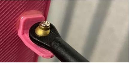
7. To secure the rudders to the rudder mounts, small hinge pins must be made. I used 1 mm servo linkage wire to create a small pin that is held in place with a 90° bend. You can use whatever you have on hand. A small amount of hot glue at the top of the pin prevents them from vibrating out.
