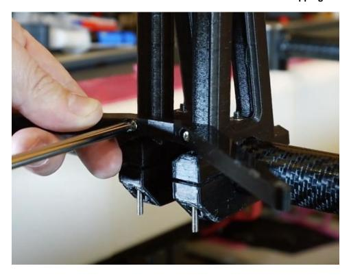
6. The rudder linkage horns are attached to each rudder using 2-part epoxy glue. The position is not important as long as they are symmetrical on both rudders. M2.5 x 27mm x 3mm Nylon Ball Joints are fitted using M2 x 10 mm machine head screws and M2 nuts. Both sides of the rudder are connected using 2.5 mm x 130 mm carbon fibre rod.
