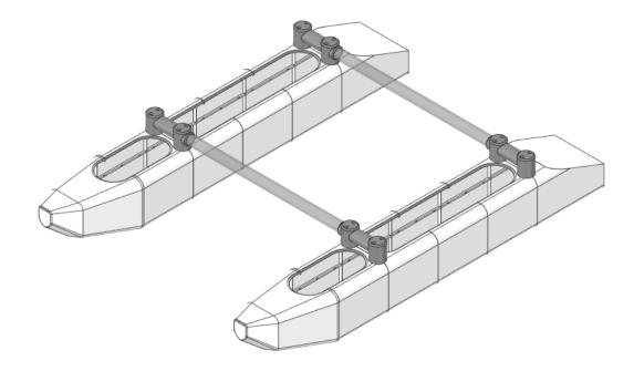
13. There are six dimples marked on the hull sections for drilling with a 3 mm drill bit to allow the hatch clips to be installed. The hatch clips are fitted with M3 x 15 mm machine head screws and M3 nylon lock nuts. The lock nuts should be tightened enough inside the hull to provide a good friction fit when the hatches are fitted. The front hatch slides into place and then the hatch clips are rotated to hold it firmly in place.
